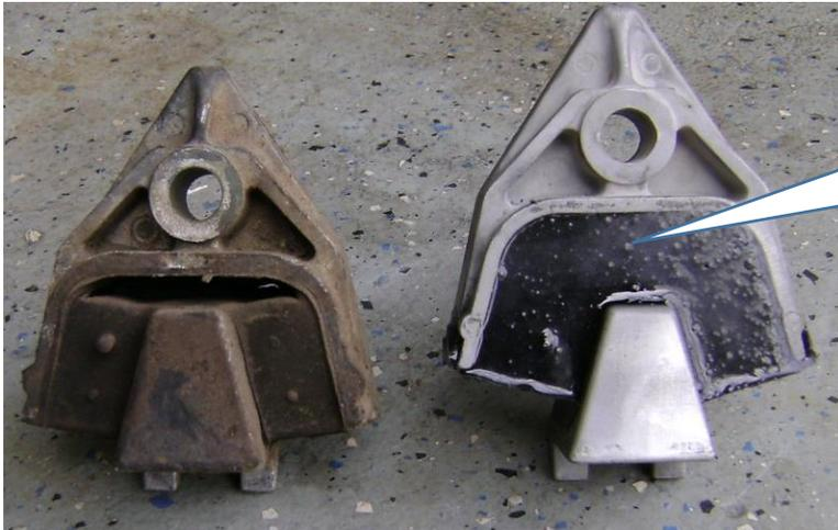
Filling in void makes isolator too stiff, not allowing for displacement
